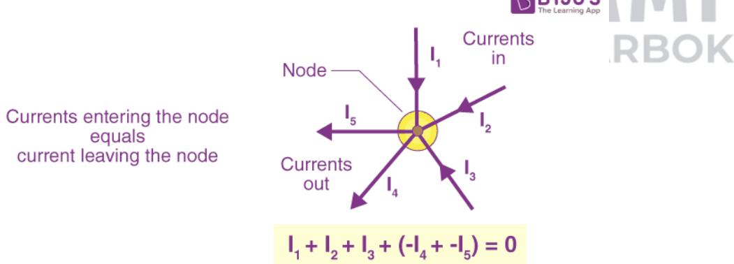
In the above figure, the currents  $I_1$ ,  $I_2$  and  $I_3$  entering the node is considered positive, likewise, the currents  $I_4$  and  $I_5$  exiting the nodes is considered negative in values. This can be expressed in the form of an equation:
