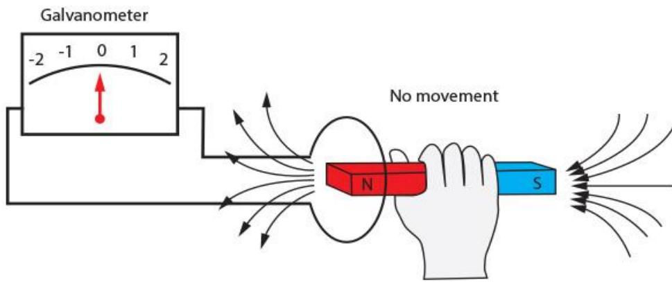
The galvanometer is moved in one direction as you go towards the loop, but moving it in the opposite direction causes the galvanometer to also move in the opposite direction, which means there is a change in the direction of the induced current in the wire.
