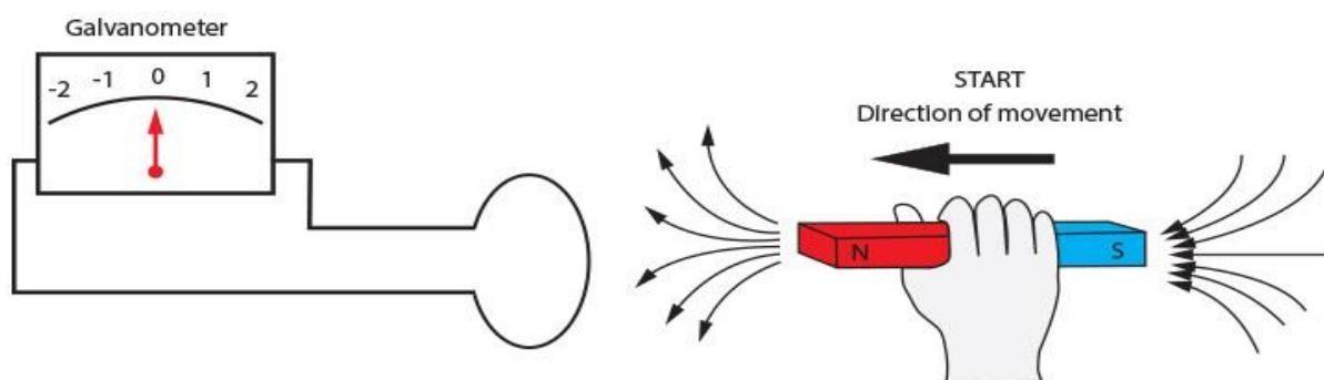
Below, a current is induced in the loop when a motion exists between the bar magnet and the loop.
