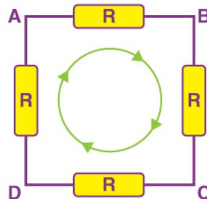
When you begin at any point of the loop and continue in the same direction, note the voltage drops in all the negative or positive directions and returns to the same point. It is essential to maintain the direction either counterclockwise or clockwise; otherwise, the final voltage value will not be zero. The voltage law can also be applied in analyzing circuits in series.
